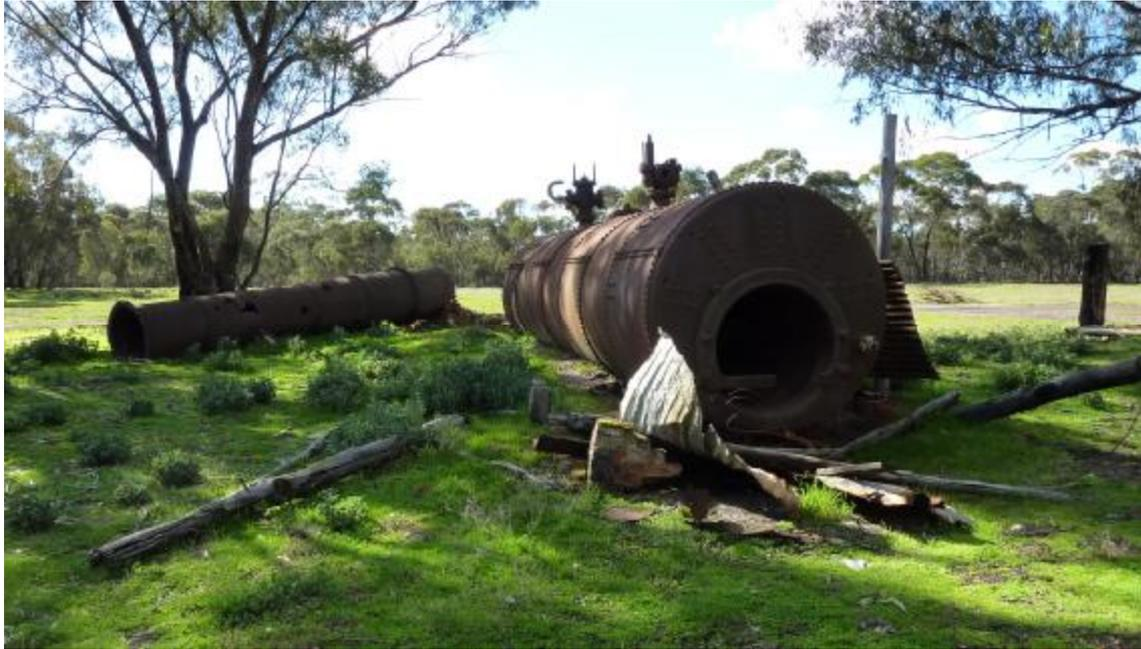
Figure 4 Former Scott's eucalyptus distillery off Scott's Road, near Neilborough. The boiler (pictured right) and the prone stack (rear left) are believed to be adapted mining machinery.
